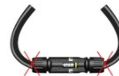
Incorrect routing of cable
